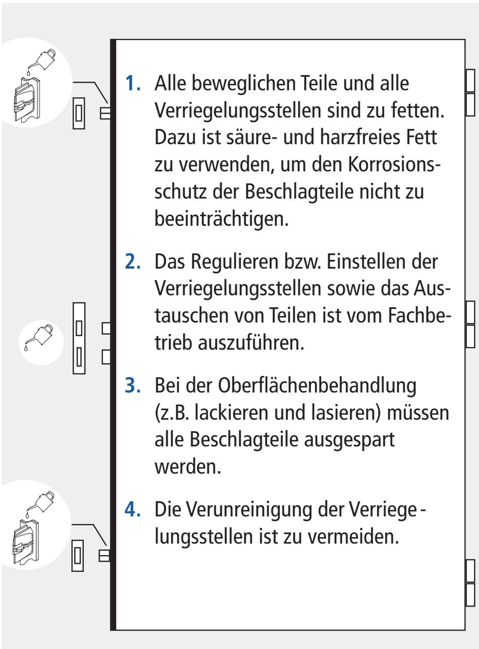
The diagram shows a vertical door lock assembly with four locking points. On the left side, there are three circular icons: the top one shows a lock mechanism being lubricated with a spray bottle, the middle one shows a spray bottle, and the bottom one shows a lock mechanism being cleaned with a brush. Lines connect these icons to the corresponding locking points on the lock assembly. A large white box on the right contains four numbered instructions.
